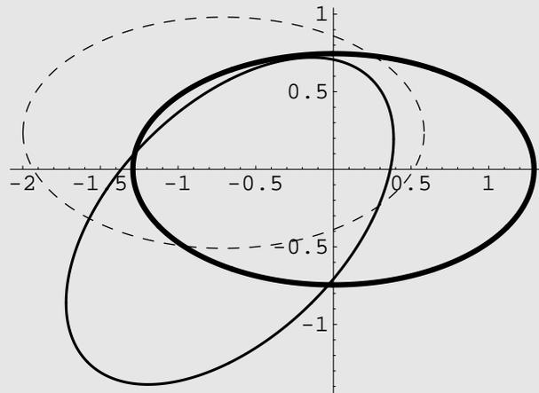
$$X^2 + 3Y^2 = \frac{5}{3}; \quad \begin{pmatrix} x \\ y \end{pmatrix} = \begin{pmatrix} \frac{\sqrt{2}}{2} & -\frac{\sqrt{2}}{2} \\ \frac{\sqrt{2}}{2} & \frac{\sqrt{2}}{2} \end{pmatrix} \begin{pmatrix} X \\ Y \end{pmatrix} + \begin{pmatrix} -\frac{2}{3} \\ -\frac{1}{3} \end{pmatrix}.$$
