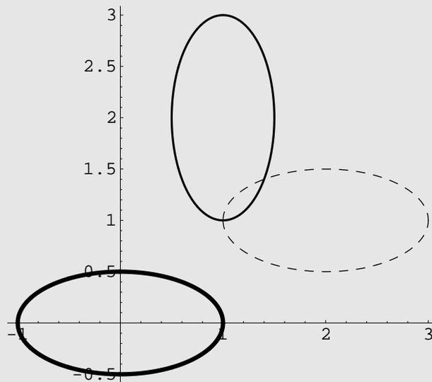
$$X^2 + 4Y^2 = 1; \quad \begin{pmatrix} x \\ y \end{pmatrix} = \begin{pmatrix} X \\ Y \end{pmatrix} + \begin{pmatrix} 2 \\ 1 \end{pmatrix}.$$
