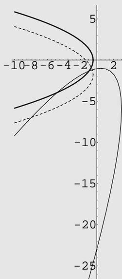
$$\frac{5}{4}Y^2 = -2\sqrt{5}X; \quad \begin{pmatrix} x \\ y \end{pmatrix} = \begin{pmatrix} \frac{1}{\sqrt{5}} & -\frac{2}{\sqrt{5}} \\ \frac{2}{\sqrt{5}} & \frac{1}{\sqrt{5}} \end{pmatrix} \begin{pmatrix} X \\ Y \end{pmatrix} + \begin{pmatrix} \frac{9}{5} \\ -\frac{6}{5} \end{pmatrix};$$
